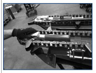
Remove the chain (in the marked phase)
