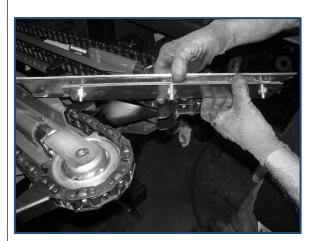
Secure the two sheet metals without tightening the screws so as to leave a gap between them
