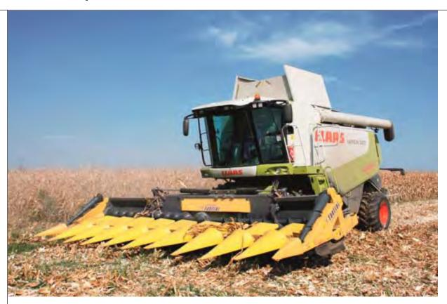
The Corn header made by Fantini S.r.l. is considered <u>Interchangeable equipment</u> according to Machinery Directive 2006/42/EC. It cannot work independently but only when attached to a combine harvester - a self-propelled machine used for agricultural harvesting purposes - from which it receives motion and all the commands.
