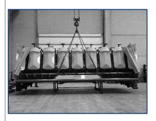
The corn header can be equipped with an iron support for transport in the vertical position.
