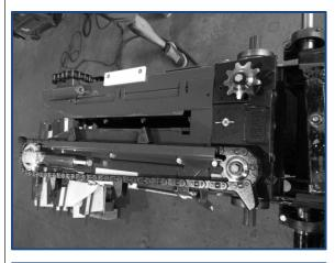
Open the right cob snapping blade until the end of its travel
