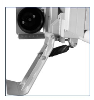
The two plates can be installed on the headers equipped with stalk choppers in order to avoid wearing down the threshing machine tyres. Without the plates, the chopped corn stalk, since it is hard and pointed, can wear down and break the tyre.
