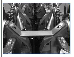
The folding version can be supplied with plates, bars or other supports to facilitate the transport.
