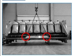
2 rear lifting points located on the vertical wall and accessible from the front;
