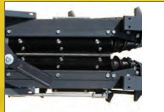
Eight sharp, heat-treated **Stalk Roll Knives** per row pull all sizes of stalks through the row unit to ensure the ear is removed cleanly.
